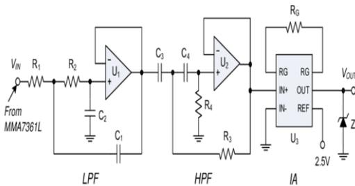
Fig.14. MEMS accelerometer interface circuit diagram.
