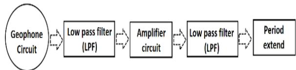
Fig.11. Geophone interface circuit diagram.
