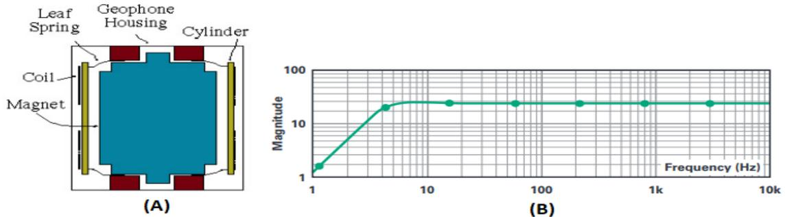
Fig.4. (A) geophone internal components, (B) geophone response (high pass filter configuration).
