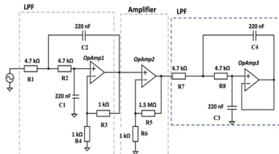
Fig.13. Geophone period expansion circuit
