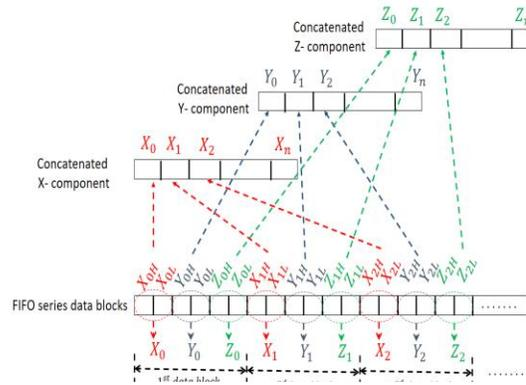
Fig.17. digital data separation and concatenation
