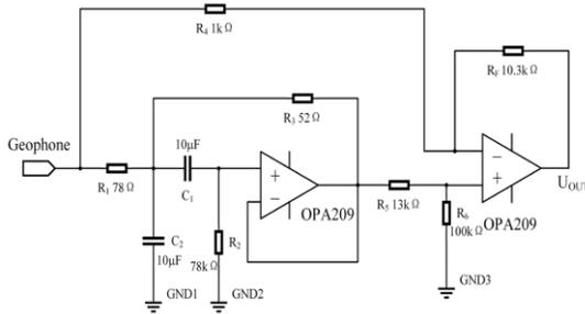
Fig.12. low pass filter and amplifier circuit for geophone
