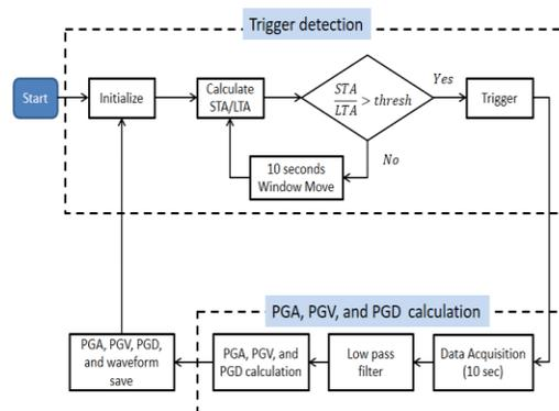
Fig.18 The event detection and processing
