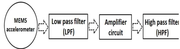
Fig.15. MEMS accelerometer interface circuit, LPF, HPF, and amplifier
