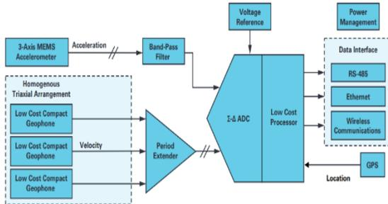
Fig.10. General block schematic of a low-cost GMMU featuring a three-axis MEMS accelerometer and three homogeneously triaxially organized geophones
