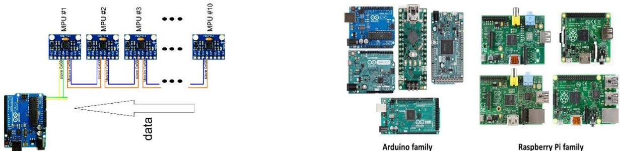
Fig 6. Multiple low-cost MEMS accelerometers connected increase measurement accuracy
