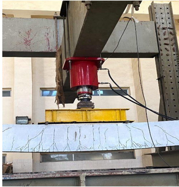
Fig. 4: Applying test load using double action hydraulic cylinder and loading frame
