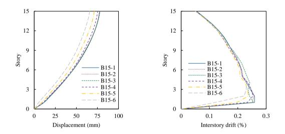
Fig. 19. Maximum story displacements and interstory drifts of the fifteen-story building configurations.
