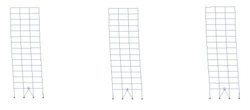
B15-4 (T = 0.79 s) Fig. 7. First mode shape of the fifteen-story configurations. B15-6 (T = 0.75 s)
