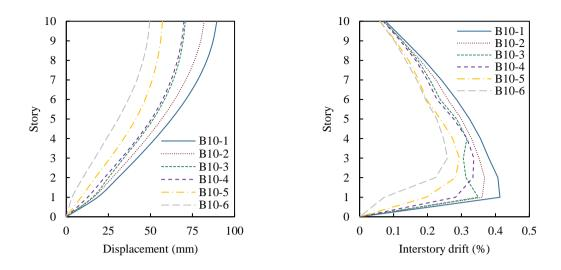
Fig. 16. Maximum story displacements and interstory drifts of the ten-story building configurations.
