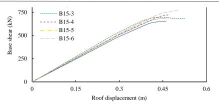
Fig. 10. Pushover curves for the fifteen-story configurations.
