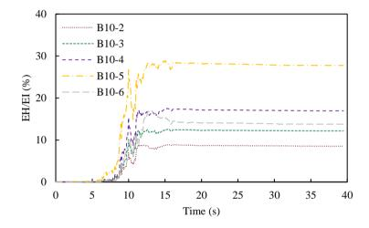
Fig. 17. Ratio of dissipated energy to earthquake input energy for the ten-story building configurations.
