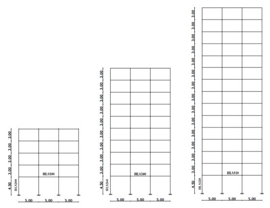
Fig. 2. Elevation view of the buildings.
