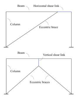
Fig. 1. Typical eccentrically braced frame.
