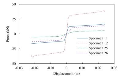
Fig. 3. Skeleton curves of shear force and shear displacement for the vertical shear links
