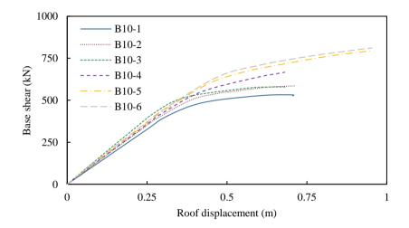
Fig. 9. Pushover curves for the ten-story configurations.
