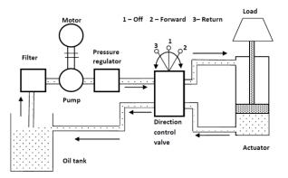
Fig.1 Components of a hydraulic system
