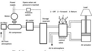
Fig.3 Components of a pneumatic system.
