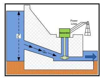
Fig. 4the hydroelectric power station
