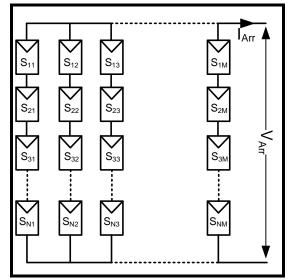
Fig. 3: solar cell array N series cell and M parallel string
