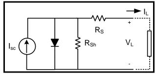
Fig. 2 Equivalent circuit for solar PV
