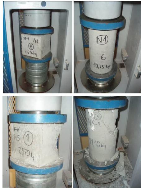
Fig. 5. Selected samples from cube and cylinder strength tests
