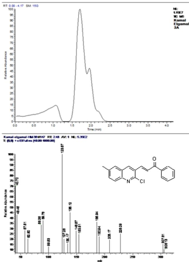
Figure 4. MS spectrum of 3a
